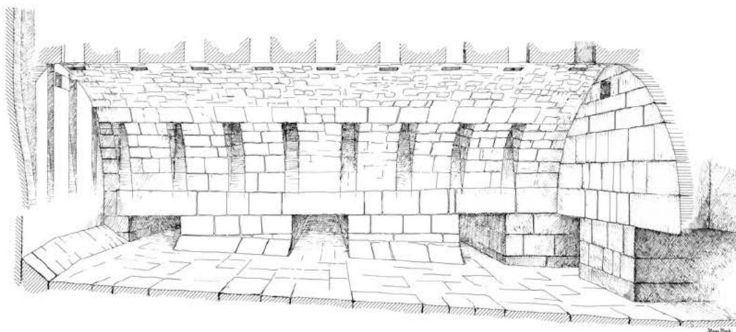
Fig. 27.5. The Latrine Complex: isometric view of the central collecting chamber, looking north.
