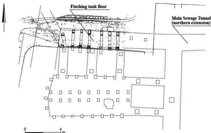
Plan 27.4. The Latrine Complex in the Hospitaller Compound: the flushing tank.
